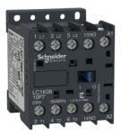
Contactor, IEC, TeSys K, 9A, 3 P, 5 HP at 480VAC, nonreversing, 1 NO auxilliary contact, 110VAC 50/60 Hz coil
